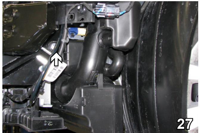
27. Reinstall the air baffle with a 6MM-1 x 45MM hex bolt, 1/4" lock washer and 1/4" flat washer on the outside. Reattach the other bolts.
