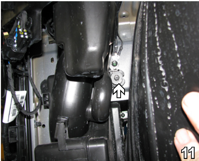
11. On the driver side, using a 10MM socket, remove the bolt from the back side of the air baffle.
