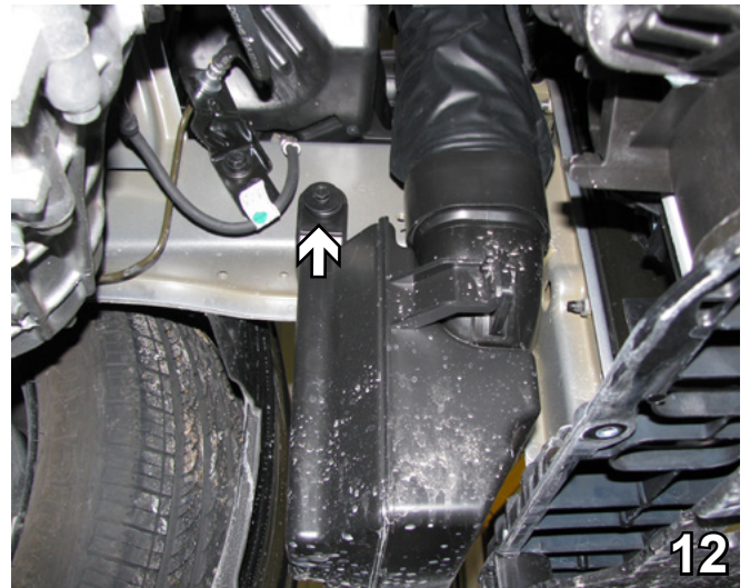
12. On the driver side underneath the vehicle, using a 10MM socket remove the bolt.
